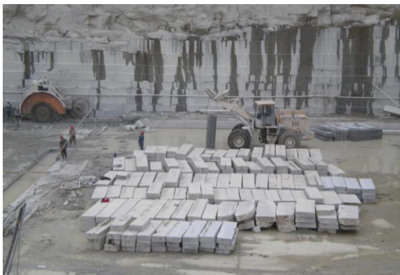
Quarrying by wire saws – an efficient method without residue.
