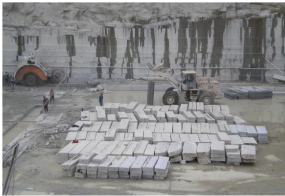
Quarrying by wire saws – an efficient method without residue.
